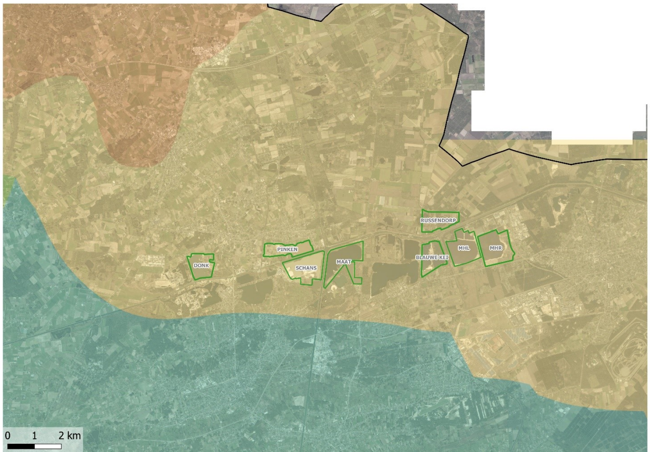
Figure 0-1 Sibelco exploitation pits of Mol Sand along the Campine Canal plotted on the geological map sheet 17 Mol, with orange: Brasschaat Formation, yellow: Mol Formation, green: Kasterlee Formation (Gullentops & Vandenberghe, 1995b). MHL & MHR Maatheide Links (Left) and Maatheide Rechts (Right). For a more recent mapping of the Brasschaat Member (now formally of the Malle Formation) see https://ncs.naturalsciences.be/paleogene-neogene/210-merksplas-formation .
